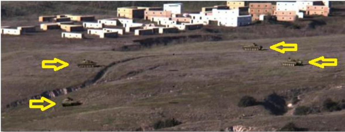
Figure 2: Virtual tanks overlaid on live range at Camp Pendleton Wiskey Range viewed via HMD.
